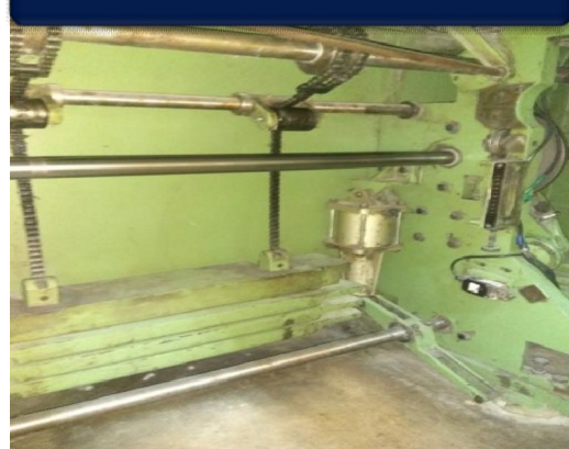
No Cone Drums after conversion
